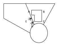
Measure Elevations at A,B,C,D,E (A+B+C+[(D+E)/2])/4 = Mean Ground Level
