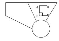
Measure Elevations at A, B, C, & D (A+B+C+D)/4 = Mean Ground Level
